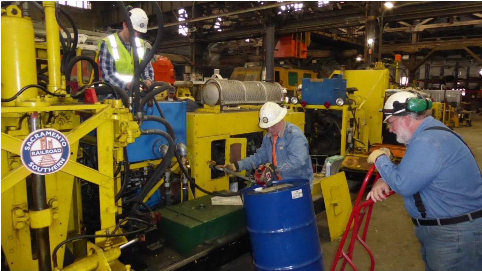
Weston, Mike H., and Frank add hydraulic fluid to the tie-shear...
